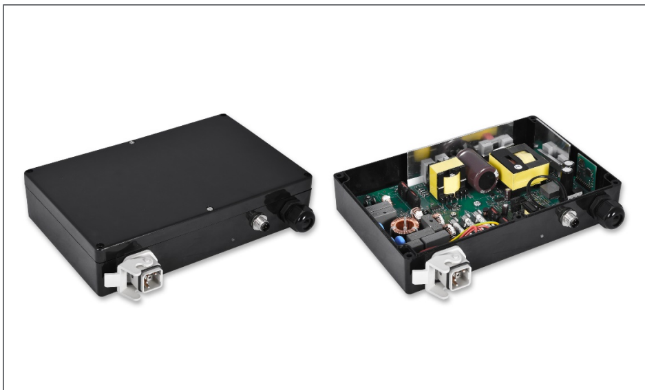
Figure 02 – PRBX ENI250A24 designed for high speed e-commerce hubs conveyers with microprocessor controller and energy recycling
