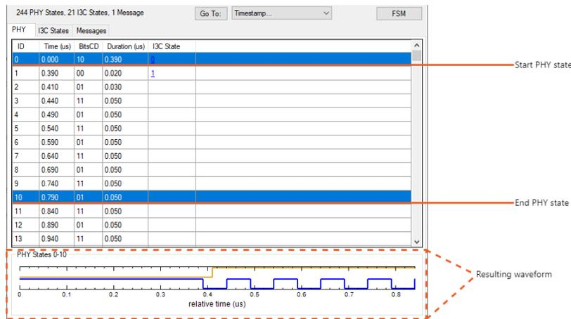
Note that the top waveform is for the SDA line and the bottom is for the SCL line.
