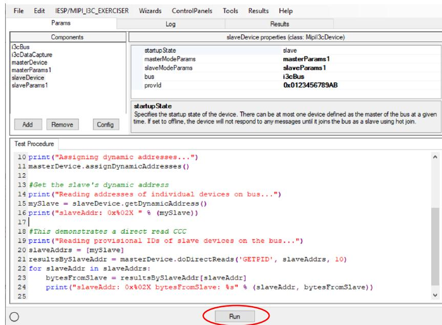
The Introspect ESP Software will execute the script. Switch to the "Log" tab, where you will see the resulting messages from your test procedure, as shown in the image on the next page. Observe that the provisional ID read back is six bytes long (each byte in the log is shown in decimal), matching the six hex bytes set previously in the slave parameters.
