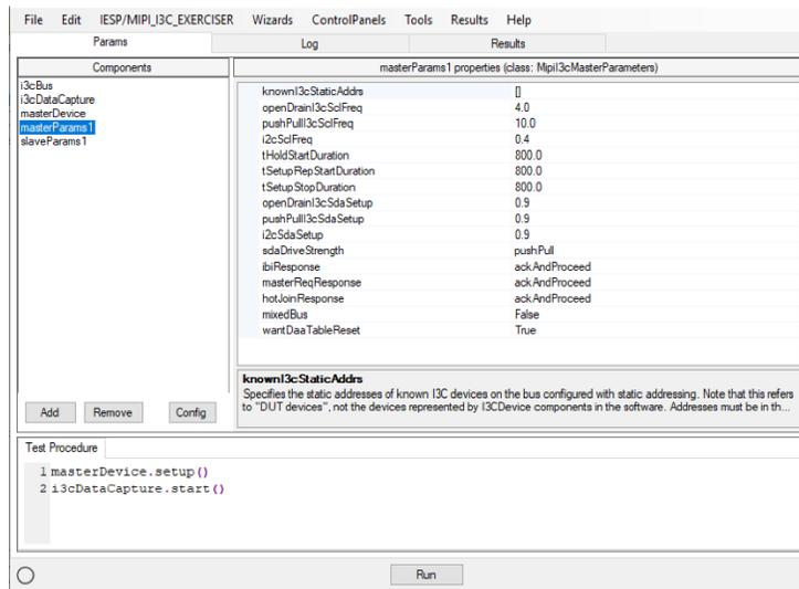
The screenshot shows the configuration window for 'masterParams1' properties (class: Mipil3cMasterParameters). The 'Components' list on the left includes i3c-Bus, i3c-DataCapture, master-Device, masterParams1 (highlighted), and slaveParams1. The 'Results' pane displays a table of parameters and their values.
