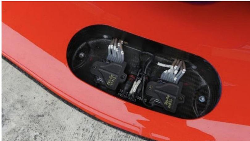
Because the aerodynamic point of interest, and point of measurement, is connected via a tube to the pressure sensor, or scanner, there can be detrimental effects in the measurement.
